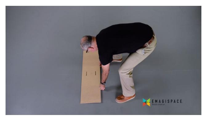
3. Insert (2) ribs into the face panel slots of the MDF Face Panel. Make sure the rib tabs are fully seated in the Face Panel slots and make sure the length of the ribs are flush with the bottom face panel. On initial assembly you may find it useful to gently tap the ribs into place using a rubber mallet.
