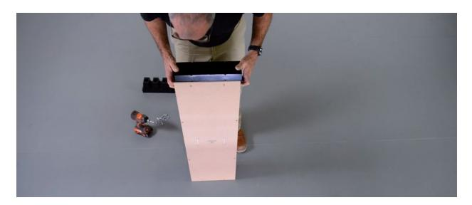
VERY IMPORTANT: BE SURE THE FACE PANELS AND BLOCK CONNECTORS ARE FLUSH AT THE CORNERS AND EDGES. ALSO, MAKE SURE THE CHANNEL CUTOUTS ARE FLUSH WITH THE RIBS. This seats the Face Panel and prevents the BLOCK CONNECTOR corners from slipping out of square.
