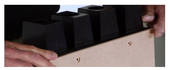
12. Hold the BLOCK CONNECTOR firmly so that it sits flush with the top and sides of the Face Panel. Insert (1) Pancake Screw through the first corner hole in the top Face Panel and drive the screw STRAIGHT IN with a square head drill/driver until the head of the screw is near, *but not* fully inserted into the countersink. Hand tighten the screw to finish. The screw will be flush with the face panel when it is fully seated. BE VERY CAREFUL TO NOT OVER-TIGHTEN.
