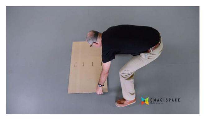
3. Insert (4) ribs into the face panel slots of the MDF Face Panel. Make sure the rib tabs are fully seated in Face Panel slots and make sure the length of the ribs are flush with the bottom face panel. On initial assembly you may find it useful to gently tap the ribs into place using a rubber mallet.
