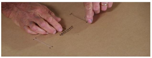
Note: It is always best to work from one side to the other, partially seating the tabs until all are seated. Once all the tabs are seated in the face panel slots, gently tap with your hand or use a rubber mallet to fully seat the tabs in the face panel.
