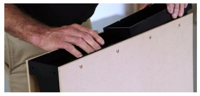
VERY IMPORTANT: BE SURE THE FACE PANELS AND CONNECTOR BLOCKS ARE FLUSH AT THE CORNERS AND EDGES. ALSO, MAKE SURE THE CHANNEL CUTOUTS ARE FLUSH WITH THE RIBS. This seats the Face Panel and prevents the BLOCK CONNECTOR corners from slipping out of square.
