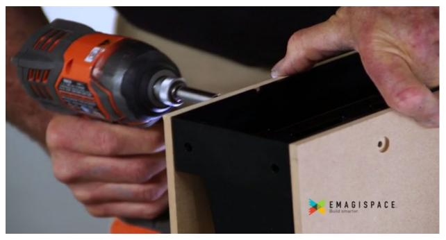
8. Repeat this process three times, for the three remaining corners of the EmagiBlock<sup>®</sup>. Secure the corners first, before securing the remaining screws.
