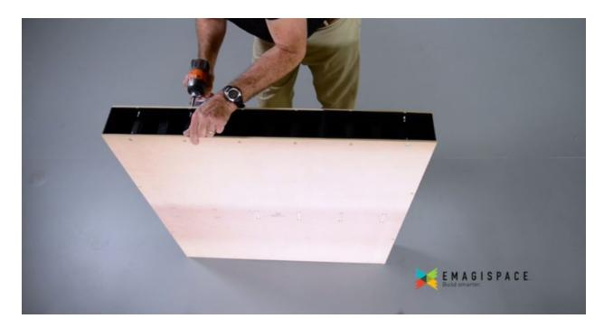
10. Grasp the EmagiBlock<sup>®</sup> on both sides, holding firmly so that the MDF Face Plates stay seated in the Ribs, and carefully flip the EmagiBlock<sup>®</sup> 180° (*Set the EmagiBlock<sup>®</sup>* on the end with the installed BLOCK CONNECTORS, and pay careful attention to keep all the Ribs seated throughout this process.)
