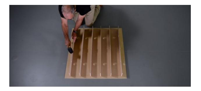
4. Place the second MDF Face Panel on top of the ribs and fully seat the tabs from each rib into the top face panel slots. Make sure the ribs are fully seated in the slots. The blocks should go together fairly easily but sometimes a tab will become misaligned making it hard to seat. In these instances, a slight wiggle will help seat the ribs. Other times, it is possible to use a nail or similar implement to help align the rib tabs with the panel slots.
