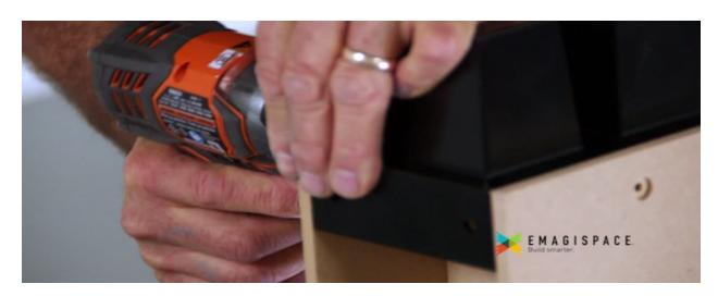
13. Repeat this process three times, for the three remaining corners of the EmagiBlock<sup>®</sup>. Secure the corners first, before securing the remaining screws.
