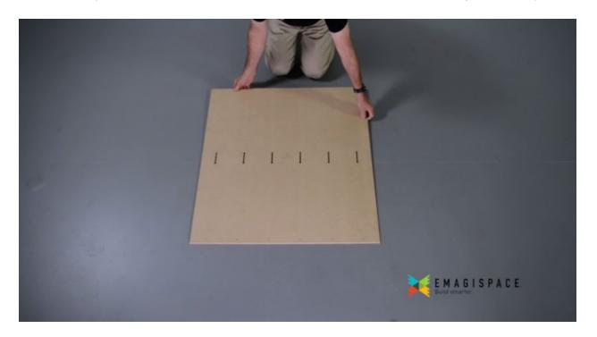
3. Insert (6) ribs into the face panel slots of the MDF Face Panel. Make sure the rib tabs are fully seated in the Face Panel slots and make sure the length of the ribs are flush with the bottom face panel. On initial assembly you may find it useful to gently tap the ribs into place using a rubber mallet.
